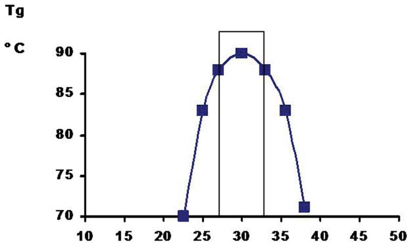
Parts by weight of hardener RS-MH137 to 100 parts by weight of laminating resin RS-M135. Heat treatment 80°C.
