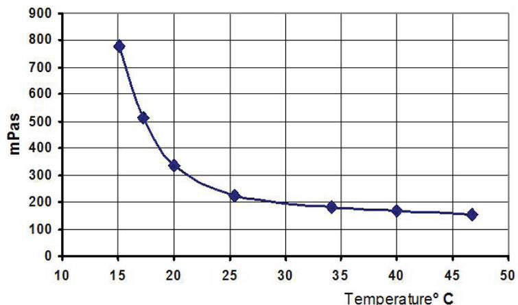
The mixed viscosity is very low, which is especially advantageous for injection and pultrusion methods. By heating the resin mass, the viscosity can be reduced further to approximately 150 mPa s at 46°C (see diagram), enabling complicated moulded parts with long flow paths to be easily injected. The temperature rise with hardener RS-MH137 remains very low up to a mould temperature of approximately 30°C, so that even parts with thicker layers can be produced at elevated temperatures.
