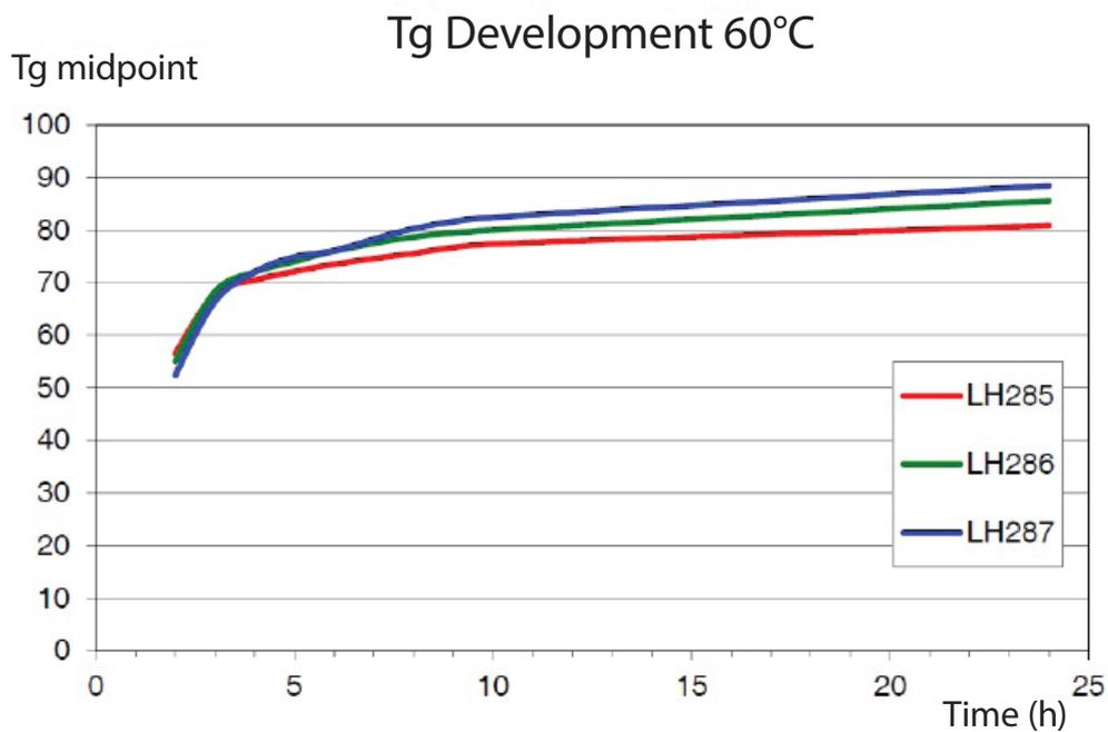
Measuring conditions for all Tg measurements: DSC, ISO 11357
